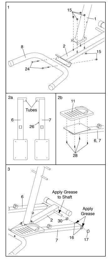
4. Apply grease to the lower shafts on the Upright (1).
